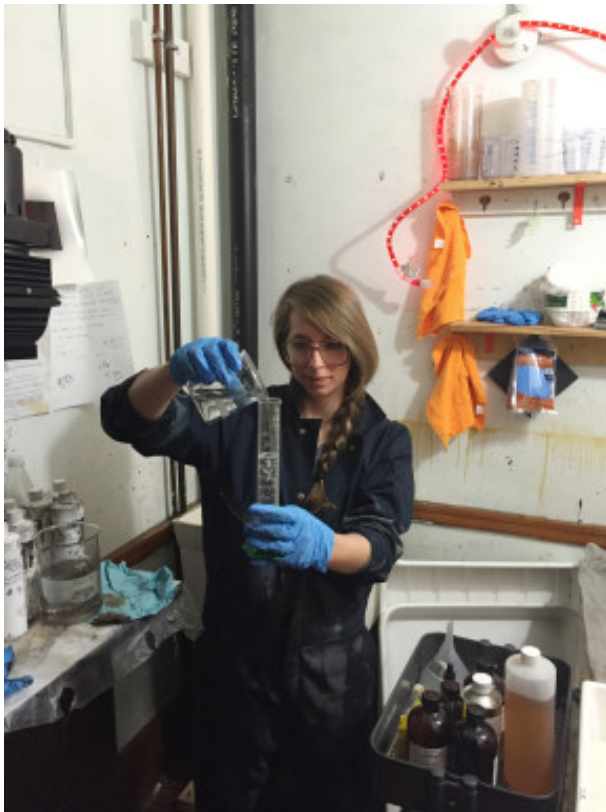
Brittany Nelson pours silver nitrate in a graduated cylinder to check the specific gravity, which indicates what percentage of silver is in the solution. MADELINE POFAHL
